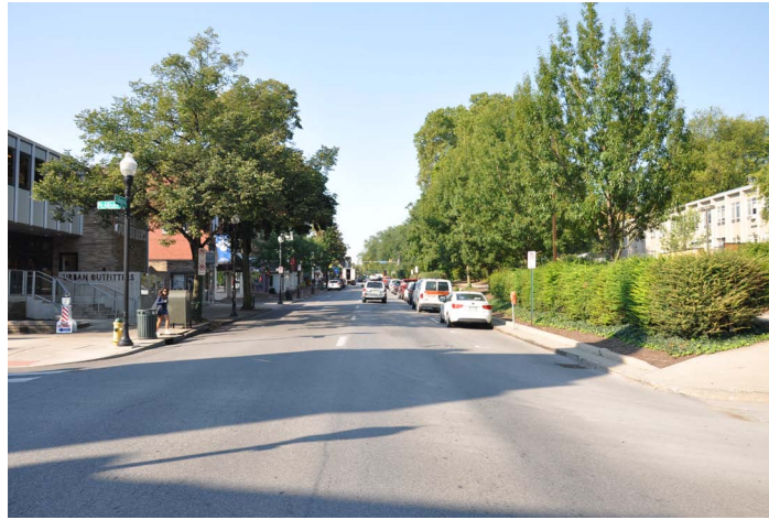
Top left: View looking west on College Avenue from the McAllister Street intersection. The existing condition along much of College Avenue includes a narrow curb-to-curb dimension; undersized parallel parking stalls on both sides of the street; inadequate sidewalk widths for typical pedestrian volumes on the south side of the street; and a shrub and fence along the north side of the street that buffers the campus walkway from the roadway, but also prohibits views to the campus.
