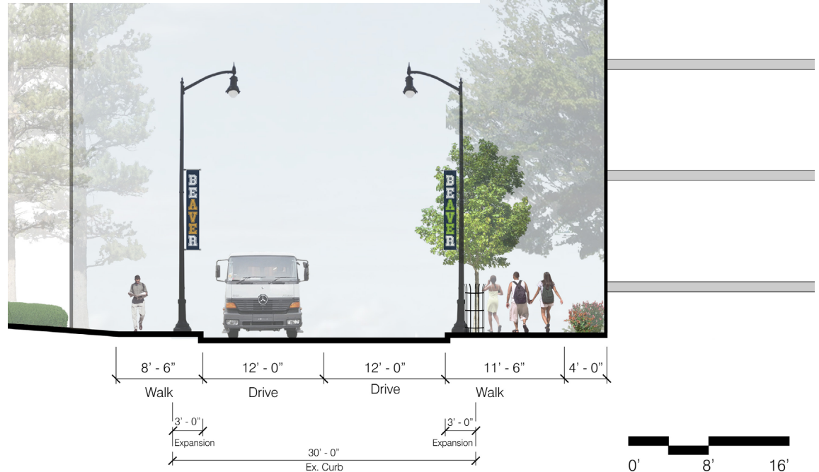
Beaver Ave. Concept Drawings: Cross Section Between Garner Street and Hetzel Street
